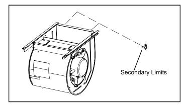
Figure 15. Secondary Limit Control
