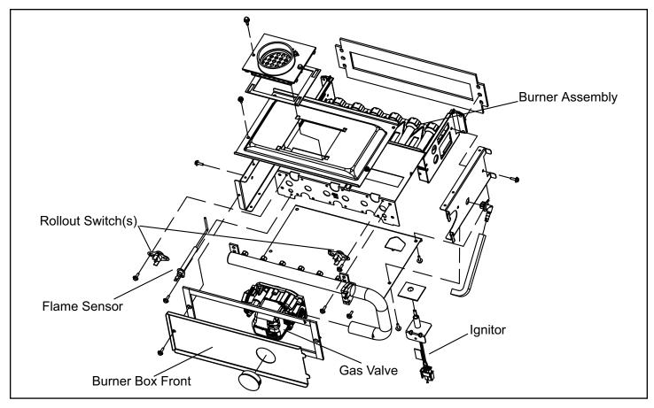
Figure 5. Burner Box Assembly
