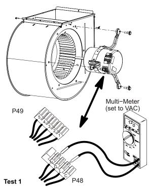
Turn on power to unit. Check for 120 volts across terminals "L" and "N" on input plug P48. If voltage is present continue to test 2. If voltage is not present, problem may be upstream of plug P48. Proceed to test 3.
