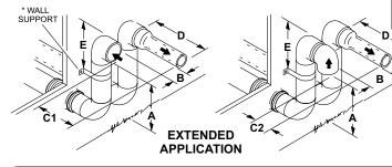
\* Use wall support every 24" (610 mm). Use two wall supports if extension is greater than 24" (610 mm) but less than 48" (1219 mm).
