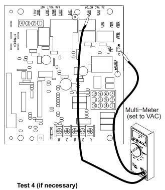
Check for 24 volts across terminals "24 COM" and "FAN" terminals on the integrated control. If voltage is present, problem is with the harness. If voltage is not present, problem may be may be with the integrated control.
