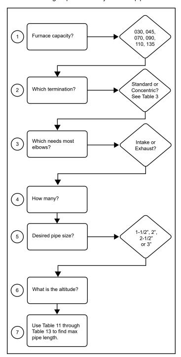
Figure 22. Vent Pipe Diameter Sizing
