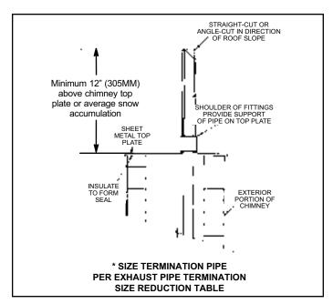
Figure 41. Non-Direct Vent Application Using Existing Chimney
