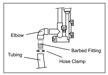
Figure 44. Field-Provided Drain Components
