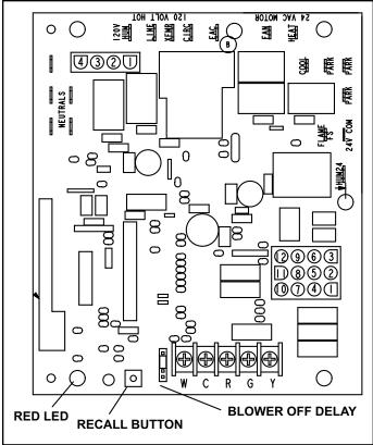
Figure 3. Integrated Control (Automatic Hot Surface Ignition System)
