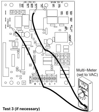
Check for 120 volts across terminals "CIRC" and "Neutrals" on the integrated control. If voltage is present, problem is with the harness. If voltage is not present problem may be may be with the integrated control.
