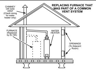
If the furnace replaces a furnace which was commonly vented with another gas appliance, the size of the existing vent pip for that gas appliance must be checked. Without the heat of the original furnace flue products, the existing vent pipe is probably oversized for the single water heater or other appliance. The vent should be checked for proper draw with the remaining appliance.
