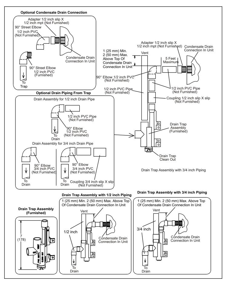
Figure 52. TRAP / DRAIN ASSEMBLY USING 1/2" PVC OR 3/4" PVC COLD END HEADER BOX WITH 1/2" DRAIN CONNECTION
