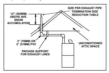
Figure 40. Non-Direct Vent Roof Termination Kit 15F75 or 44J41)
