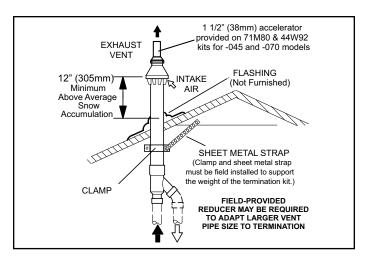
Figure 36. Direct Vent Concentric Wall Termination 71M80, 69M29 or 60L46 (US) 44W92 or 44W93 (Canada)
