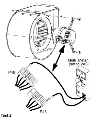
Switch thermostat to CONTINUOUS FAN MODE. Check for 24 volts across terminal "C" on input plug P48and speed tap used for continuous fan. (1, 2, 3, 4 or 5) on input plug P49. If 24 volts is not present problem may be up stream of plug P49. Proceed to test 4.
