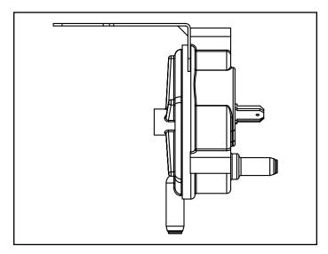
Figure 10. Pressure Switch
