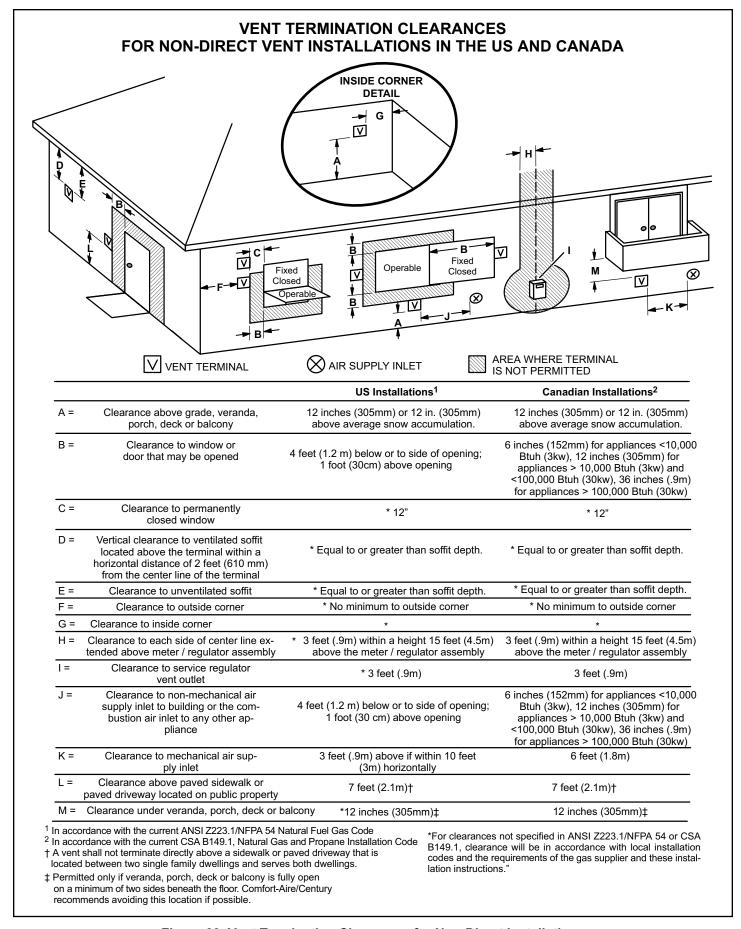
Figure 39. Vent Termination Clearances for Non-Direct Installations
