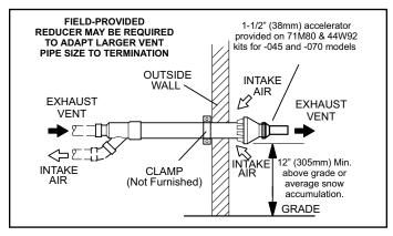
Figure 37. Direct Vent Concentric Wall Termination 71M80, 69M29 or 60L46 (US) 44W92 or 44W93 (Canada)
