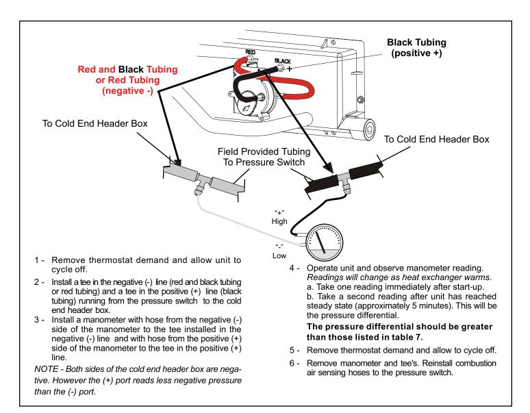
Figure 11. Measuring Pressure Differential
