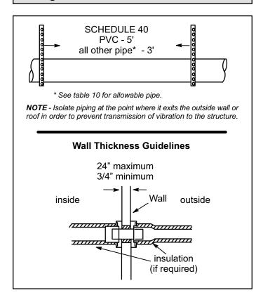
Figure 19. Piping Suspension Guidelines
